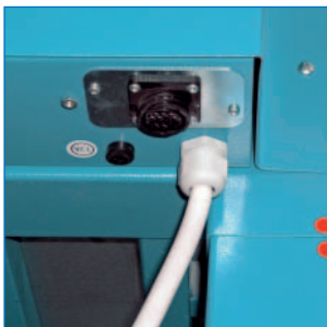
Control unit connector and micro-fuse easily accessible
